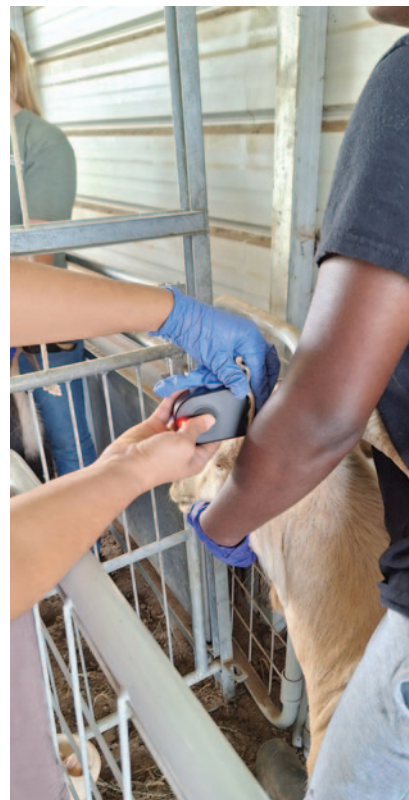
Figure 2: Handheld BIA device for impedance analysis
